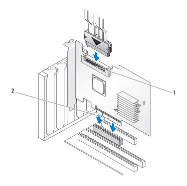
1 SAS x4 internal connector 2 PCI-E connector
